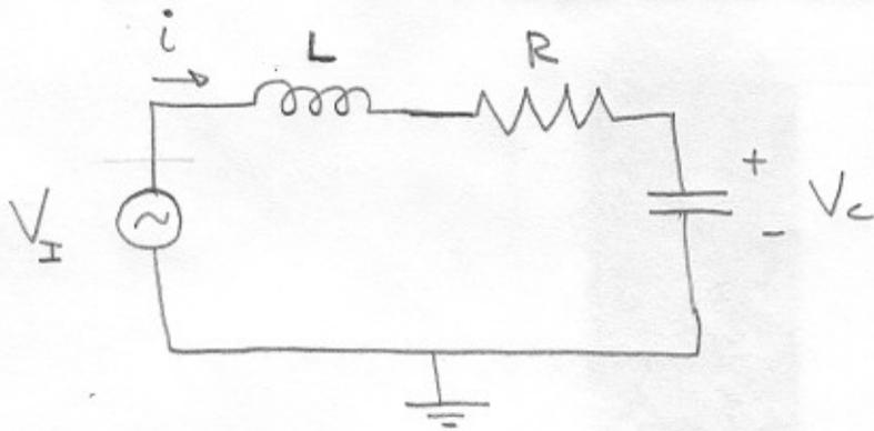
The voltage of the capacitor, resistor, and inductor must equal the voltage of the input.
