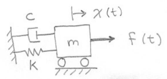
It can be shown that the equation of motion of the system is given by :
